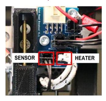
5. Replace the zip tie in the bed probe body and retain the sensor and heater wires in the zip tie. Route the wires as shown.
