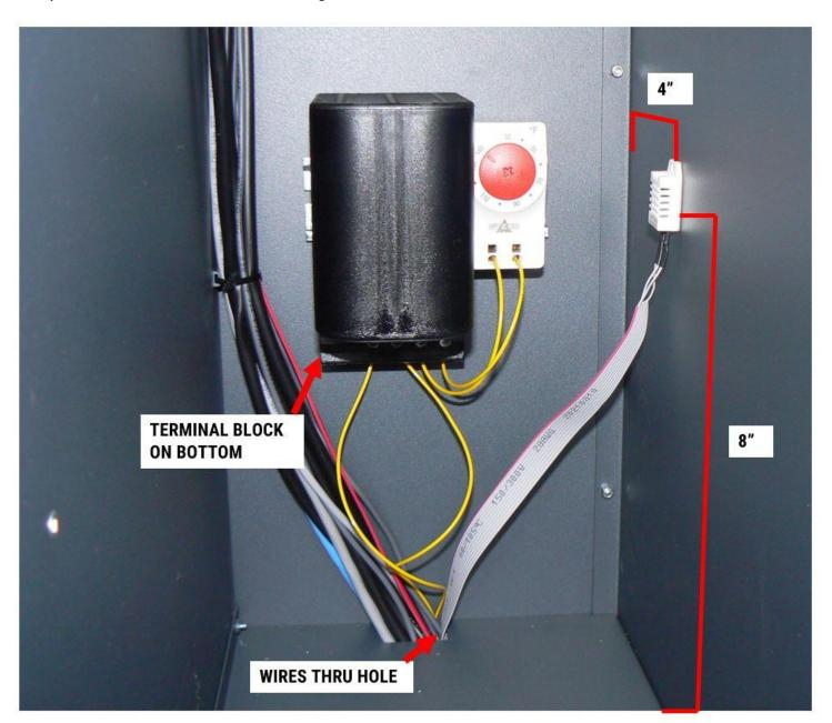
11. In the electronics bay, locate the matching yellow wires and connector. Remove the blank connector if it's present. Plug the connector in.
