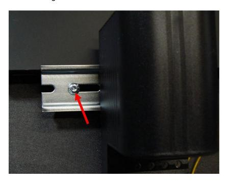
4. In the back wall of the filament bay you will see 2 holes in the sheet metal. Insert the screw through the hole and put a washer and nut on the back. Get it finger tight.
