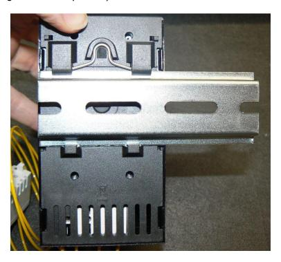
3. Insert 1 of the 2 screws through the DIN rail.
