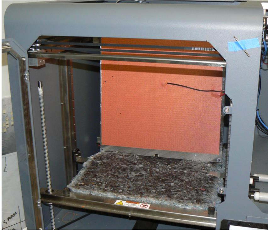
6. Remove the insulation so you can see the wing screws.
