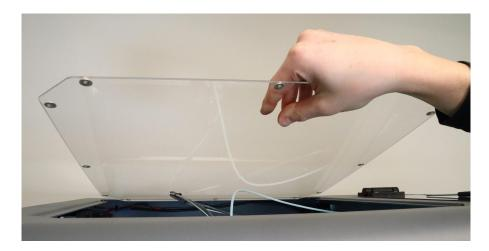
To reinstall, simply drop back into place and make sure it sits flush with the outside face of the chassis. The magnets go out the **outside** (aka top) face of the window
