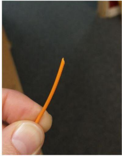
5. Feed the end into the extruder, through the inlet guide, over the wiper, over the monitoring wheel, and into the liner. Gently push until you feel it bottom out.
