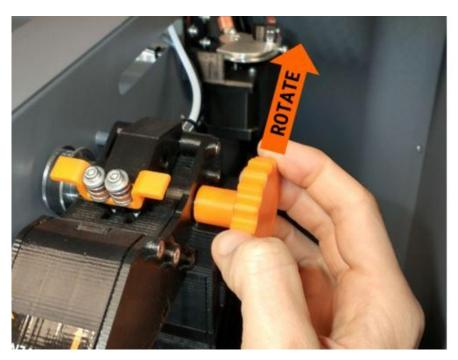
7. Continue to turn the manual advance wheel until you see the filament protrude into the bowden tube at the exit of the extruder. You need to see 1.5-3 inches protruding into the tube.
