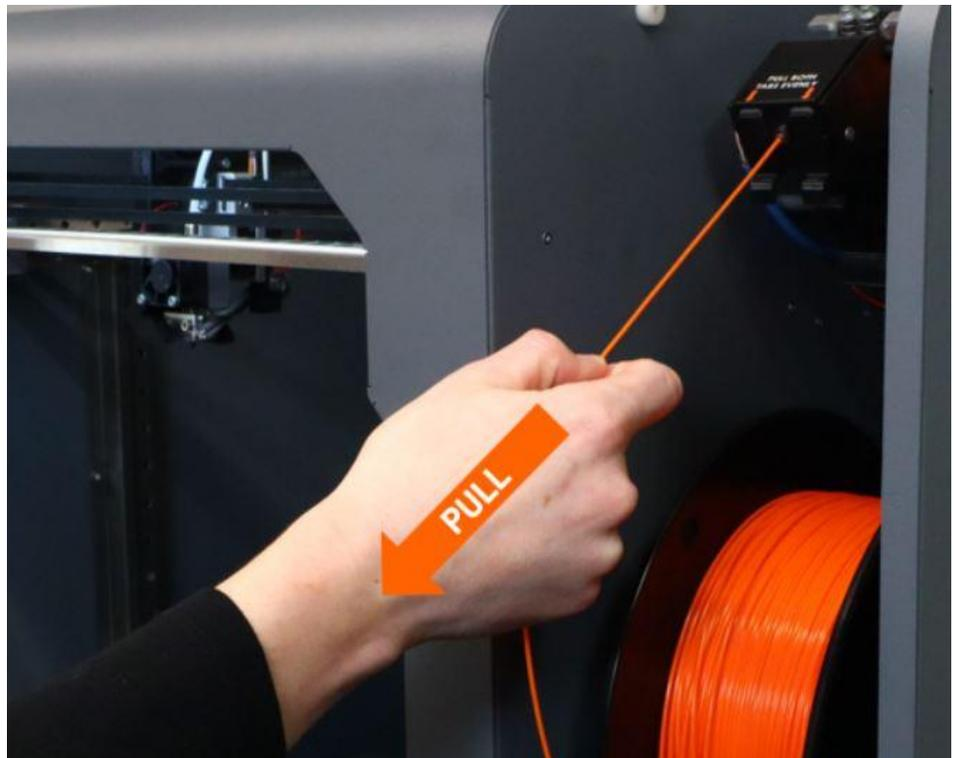
4. Spin the spool in reverse to wind up the length of filament that was ejected from the extruder. Then tuck the end of the filament into the side of the spool; most spools have small holes for this purpose.
