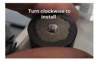
2. The bushing is fully installed when it stops turning. The bottom face of the bushing may have a small gap between it and the bed substrate. **THIS IS OK**.
