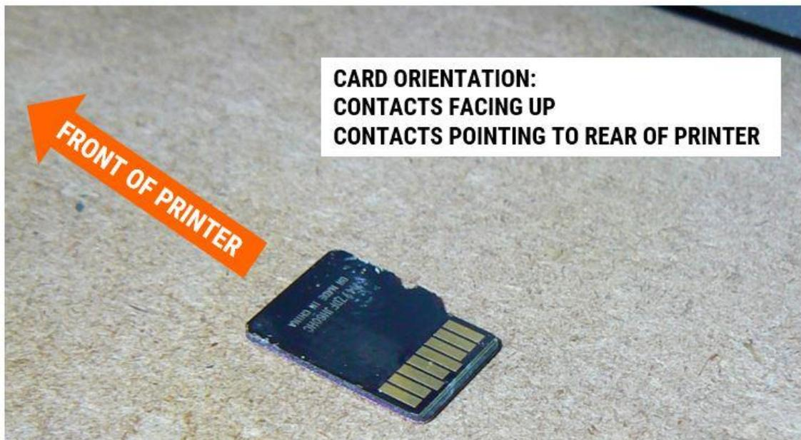
2. Position the card centered on the ribbon cable connector. The card slot is on the bottom of the PCB, so aim the card underneath the PCB.
