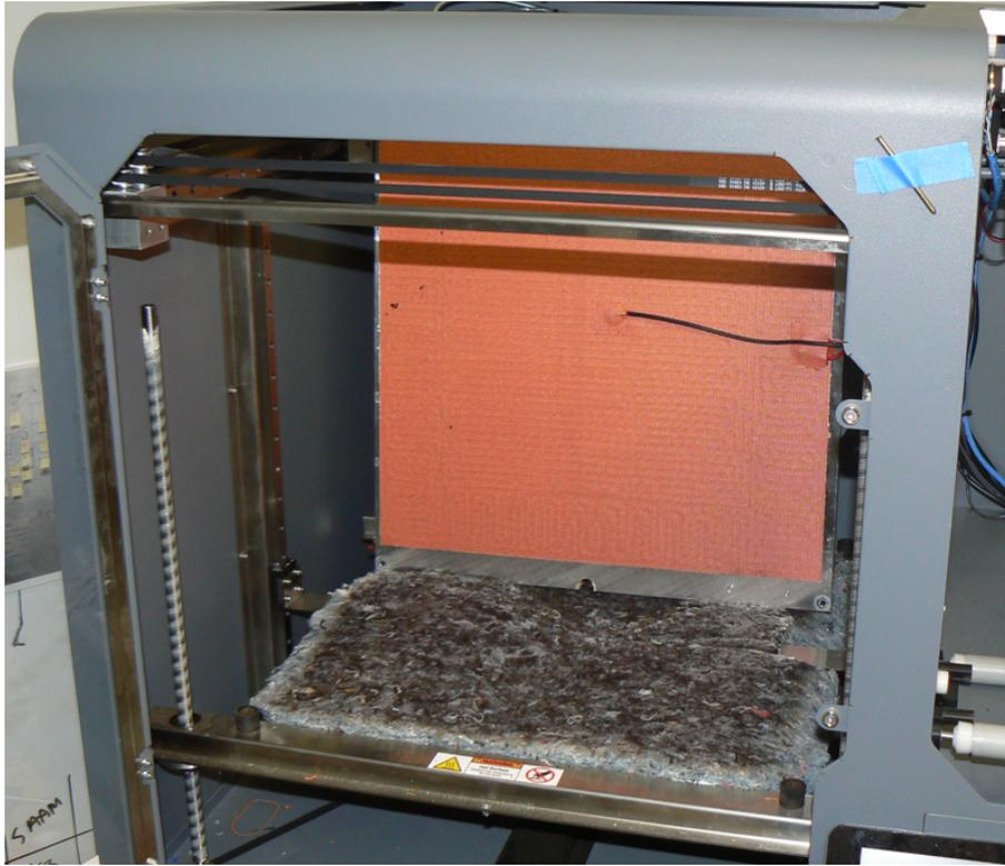
10. Use rubbing alcohol to clean an area on the heater next to the existing sensor, and where the wire will lay. Wait for it to dry.
