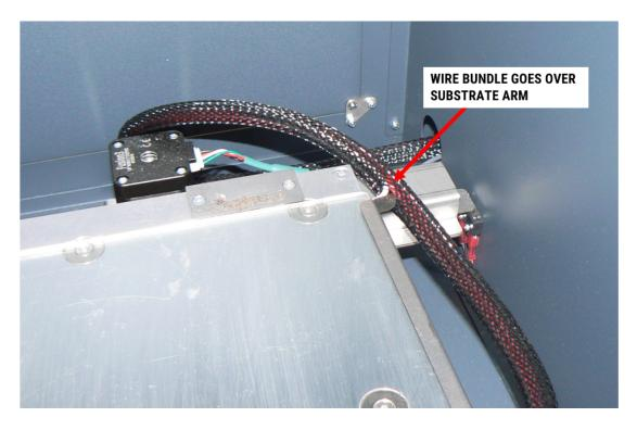
5. Route the wires through the feed-thru hole into the electronics bay.
