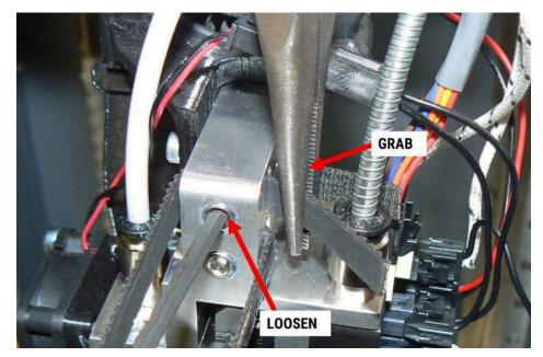
4. Relieve just enough tension on the belt to slip the belt off of the X or Y motor pulley.
