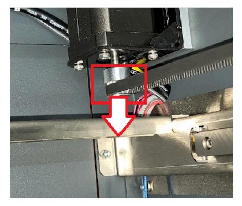
5. Tighten the set screw to keep the belt in place until the new motor is installed.
