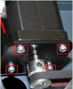
4. Once the motor is free from the mount, remove the pulley off the motor shaft.
