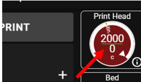
If the open circuit is intermittent, you might see this error, but when you check on the printer later you see a "real" temperature on the screen.
