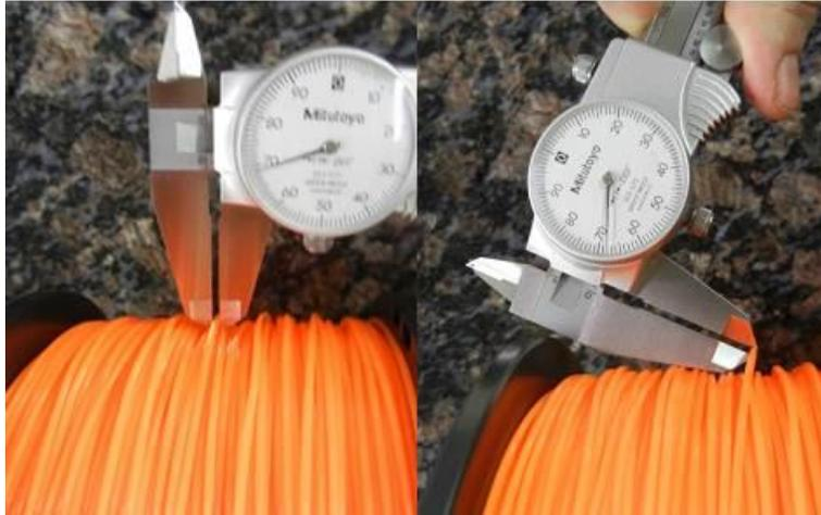
Figure 61: Measuring Filament Diameter
