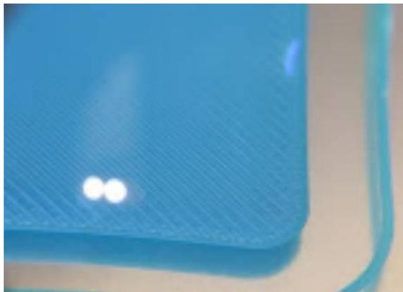
*Figure 39: First Layer is Correct*
