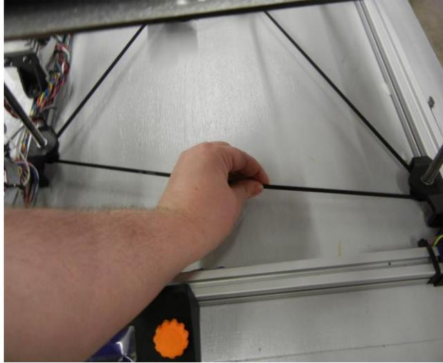
*Figure 11: Moving the Z Axis by Hand*
