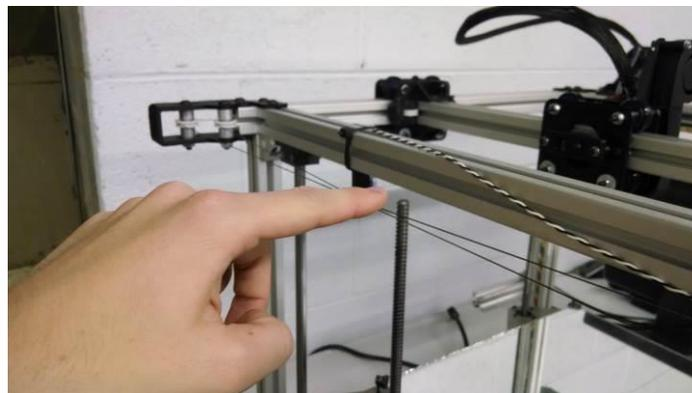
Figure 44: Checking XY Drive Cable Tension
