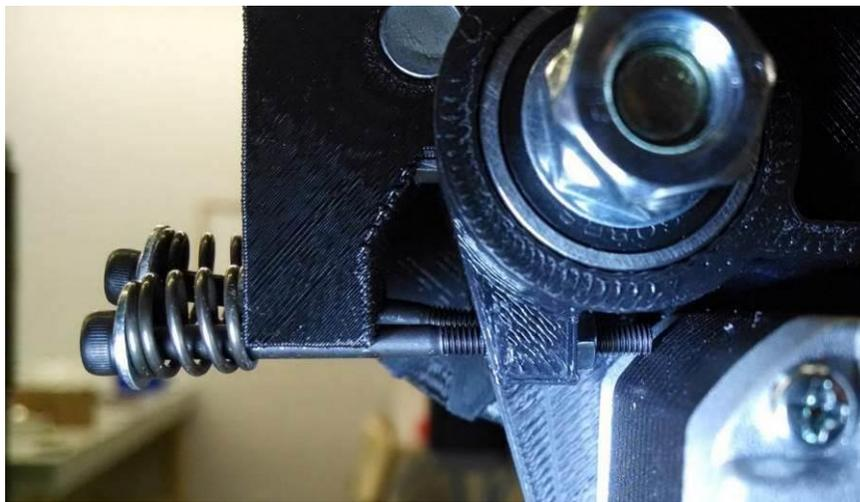
*Figure 41: Tips of Bolts Bottomed Out on Motor*
