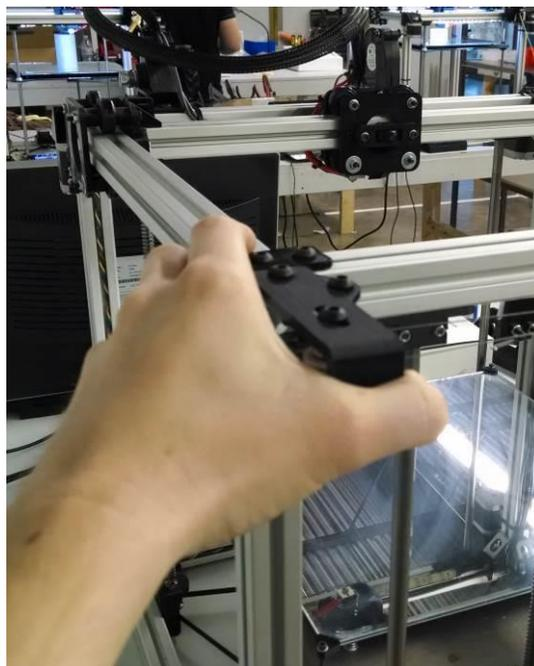
*Figure 46: Re-aligning Idler Bracket*
