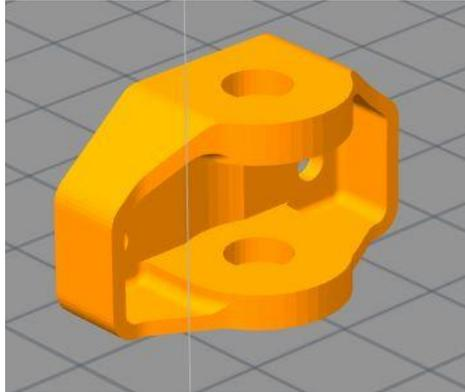
In the example shown above, we have satisfied our criteria for a large face to sit on the build plate. However, the entire upper flange is unsupported and will not print properly without support structure.
