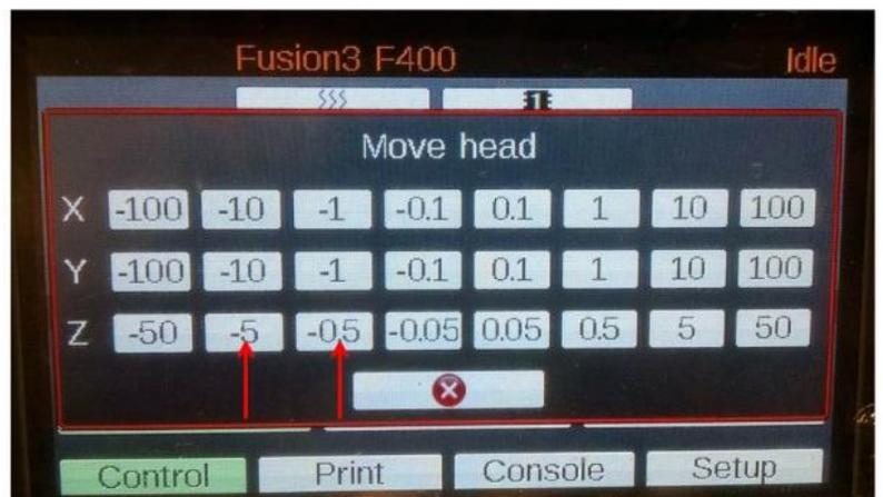
Once the gap gets small use the “-0.05” button to go up in very small increments until you have just a tiny gap between the nozzle and the bed. It can help to shine a light on the wall behind the nozzle like you see in the pictures below.
