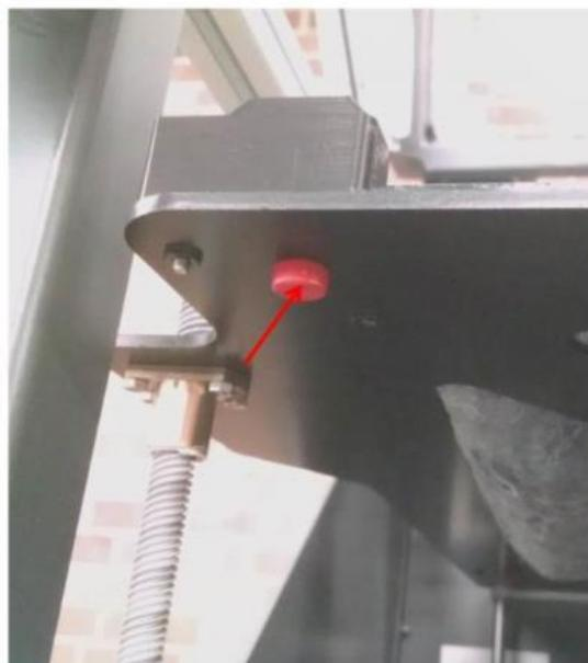
Turning the thumbscrew **counter-clockwise** will **lower** the bed corner. And turning it **clockwise** will **raise** the bed corner.
