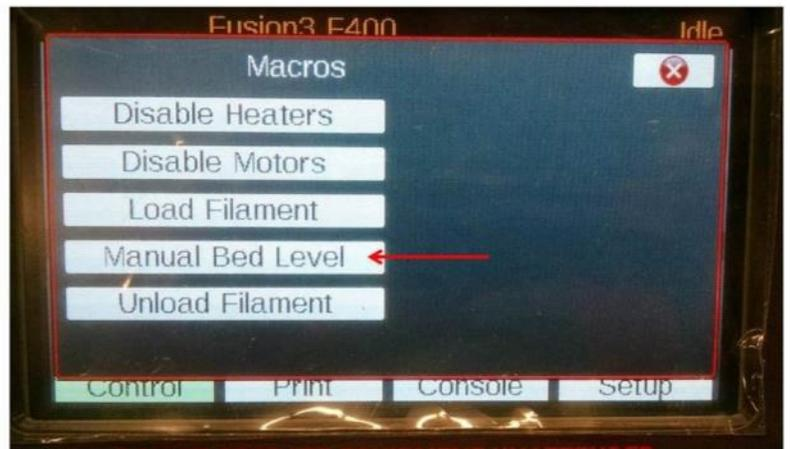
At the end of this macro the head will be positioned in the middle of the bed about 10 mm away from it, with the X and Y motors disabled (so you can move the head around by hand).
