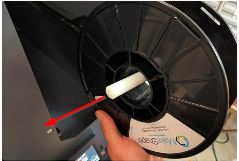
2. Orient the spool so that the filament pays off the front underneath the spool.
