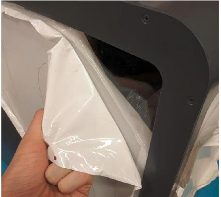
2. Remove the protective film from the LCD.
