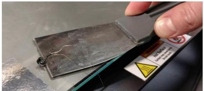
3. Allow the bed to cool to at least 45°C. Spray water onto the bed using the supplied spray bottle. Let it soak for at least 15 seconds. The glue will turn purple again.
