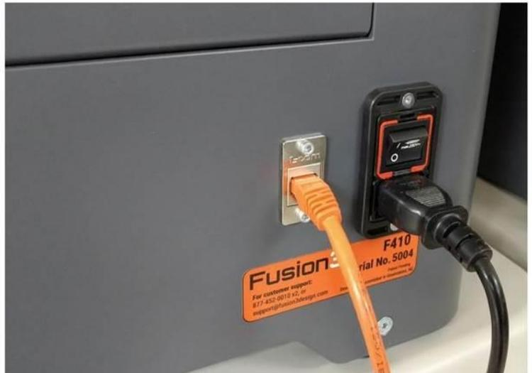
5. Power on your printer using the power switch. Wait 3-5 seconds for it to boot up.
